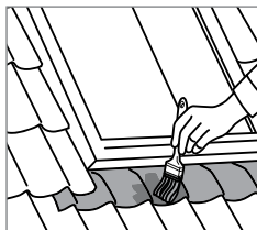
Sealing of coverings for skylights.
